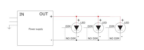
Remark: In case of non-dimming connect the DIM cable to the negative
